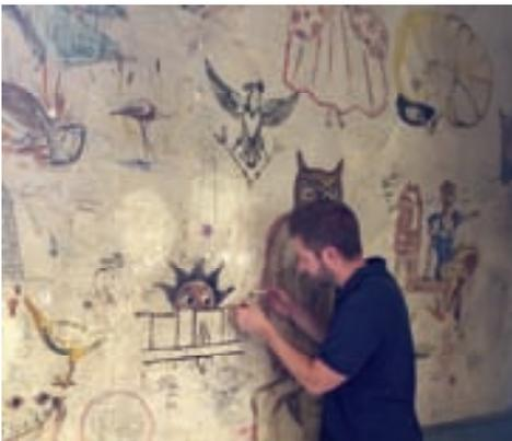
B. R. Howard & Associates art preservationist tests various products to determine which one would be best for consolidating paint that is peeling back to the plaster.
