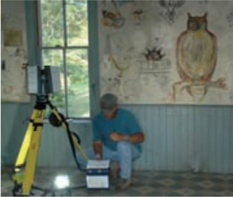
Technician sets up Leica 3D Laser Scanner to scan kitchen walls, floor and ceiling to create a historical record of the artwork before preservation began, courtesy of RIKORE, Inc.
